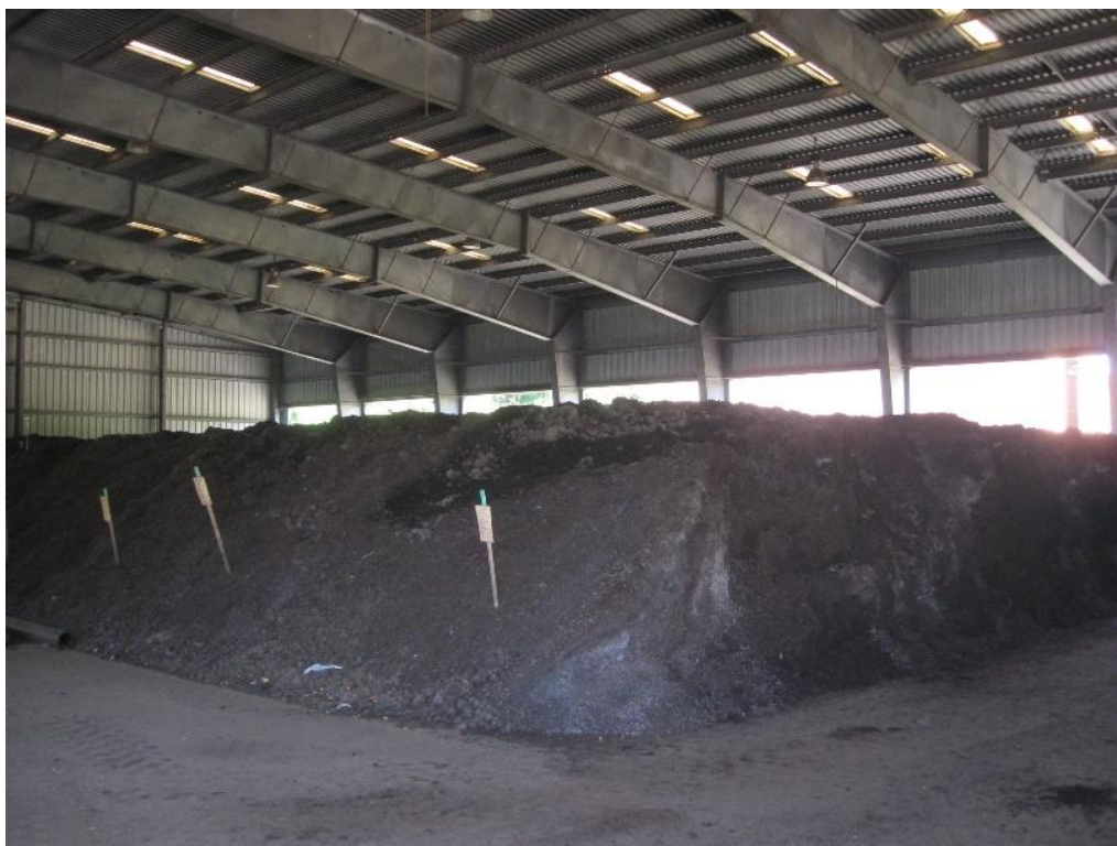
FIGURE 3-1: COVERED AERATED STATIC PILE
