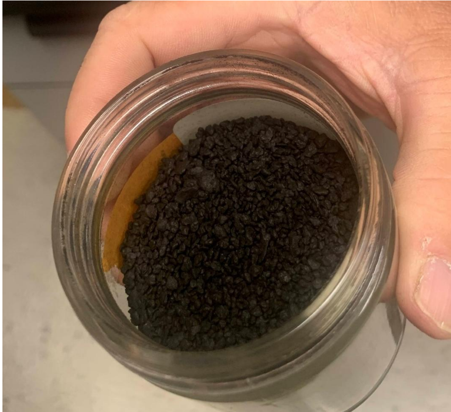
FIGURE 3-6: WILSONVILLE WWTP FINAL PRODUCT
